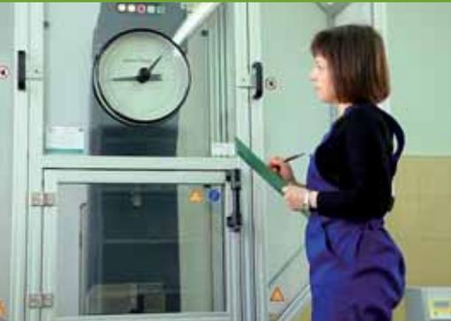
**Charpy's hammer** with a cooler for samples. Impact strength tests are performed in our laboratory in temperature range from  $-70^{\circ}\text{C}$  up to  $+200^{\circ}\text{C}$ .
